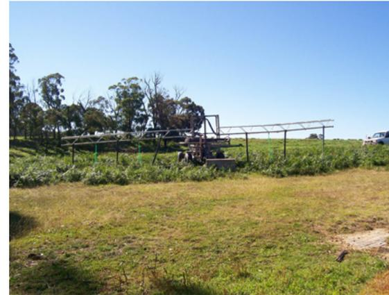
Travelling drip irrigators can apply effluent evenly at low rates.
