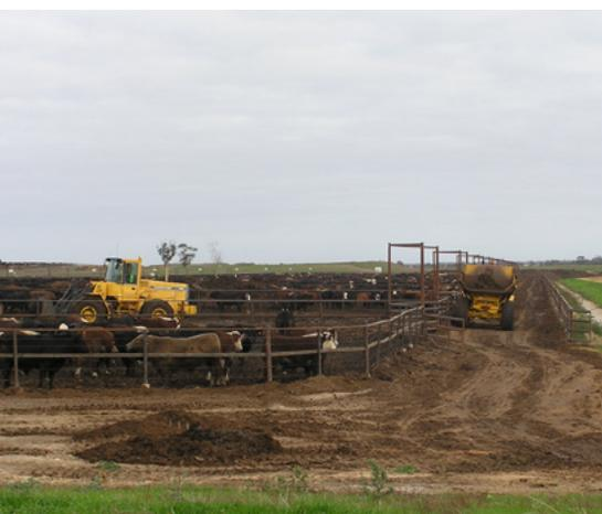
Front-end loader taking manure to an articulated dump truck during pen cleaning operations.
