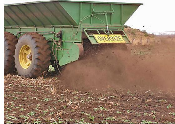
*Most spreaders need a minimum rate of 5 t/ha for even spreading.*
