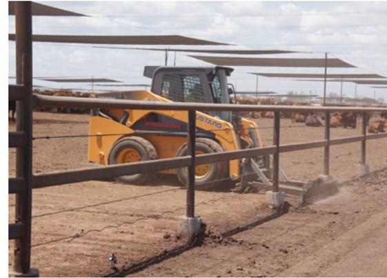
*Manure being removed by a under-fence pusher mounted on a bobcat.*
