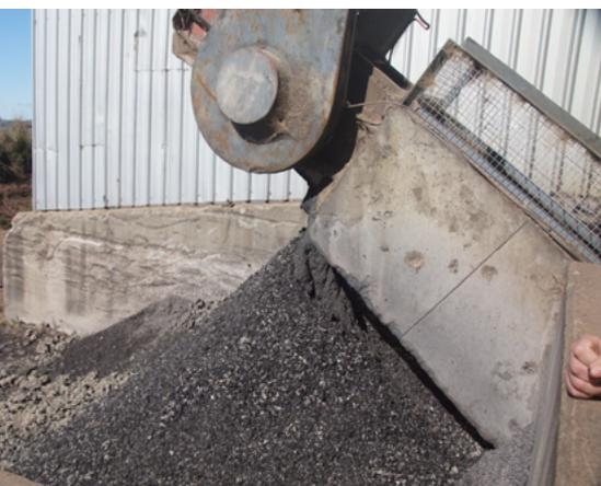
Ash produced by a coal-fired boiler.
