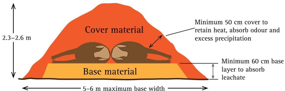
Figure 2.2 Placement of carcasses side-by-side for composting
