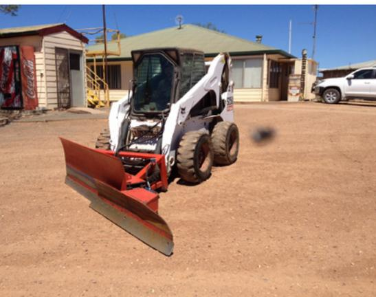
Slider blade for removing manure from under fencelines, along aprons, around shade posts, and from drains and lanes
