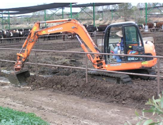
Excavator being used to clean manure from behind and underneath a fence above a drain.
