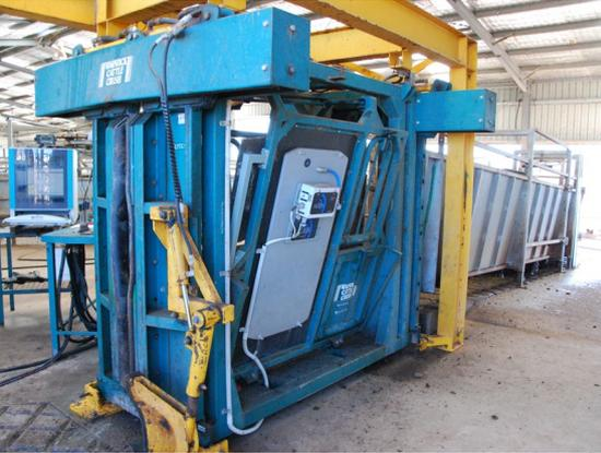
Hydraulically-operated crush with multiple features.
