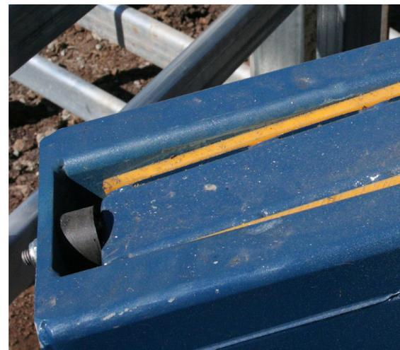
*Wear pads reduce wear, and rubber stoppers reduce noise, shock and fatigue.*
