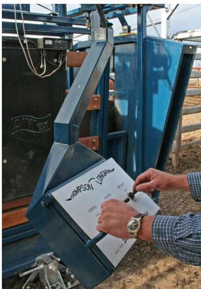
Operating console for a pneumatically-operated crush.
