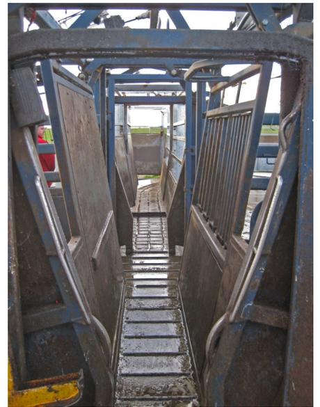
*V-opening crush – looking back into lead-up race.*
