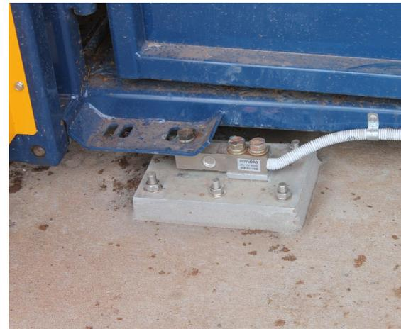
*Crush mounted on load cells for weighing.*
