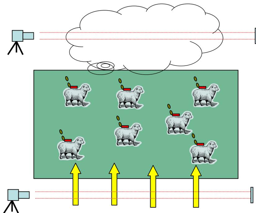
Figure 1: Schematic showing placement of instruments I1 and I2 in relation to experimental enclosure for animals and the predominant wind direction; tracer gas canisters located on animals.
