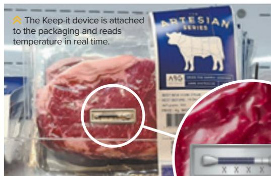
▲ The Keep-it device is attached to the packaging and reads temperature in real time.
