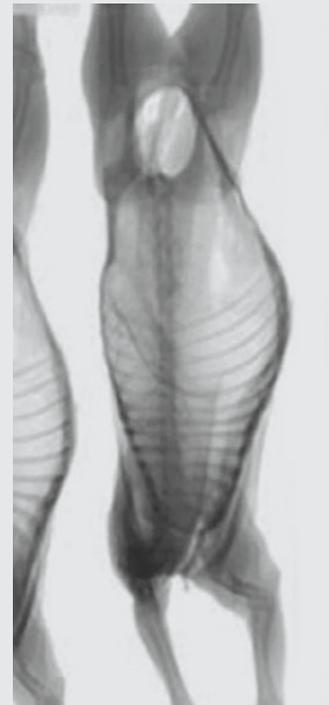
👤 DEXA device scan of a lamb carcass.
