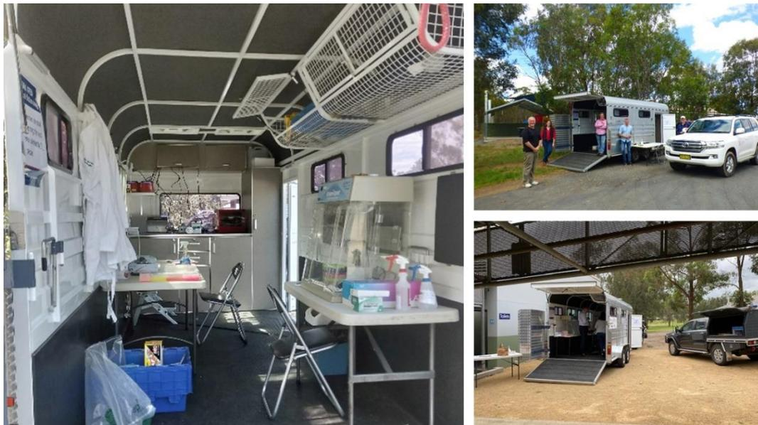
**Figure 36. Mobile 'laboratory' containing molecular testing platform for on-site sample processing and analysis. This mobile facility was used on-site co-located to a commercial feedlot in 2020.**
