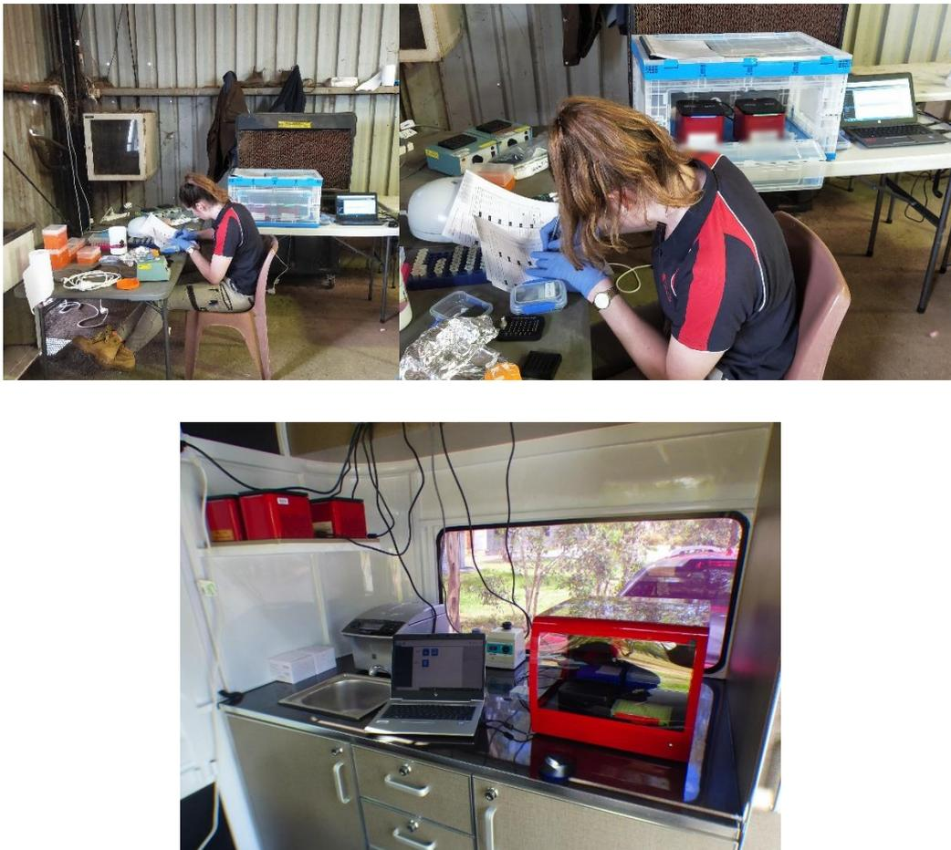
Figure 34. Top panels: Mic thermocycler being used directly in the induction facility. Bottom photograph Mic thermocycler x4 (top left) and Myra liquid handling x1 (bottom right) platforms located in the mobile laboratory shown.
