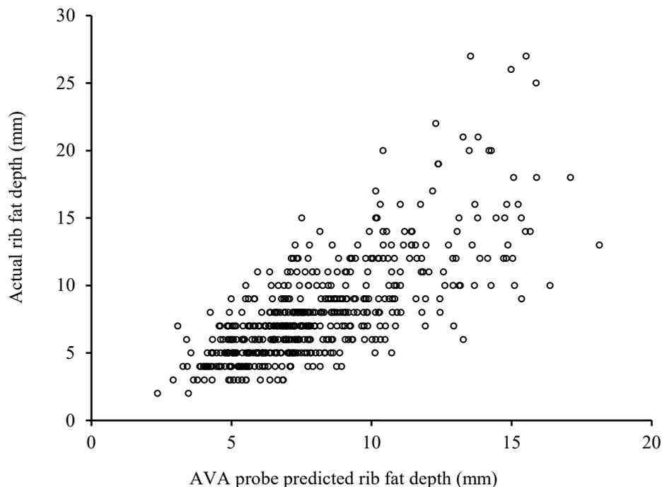
**Figure 3** The association between actual and AVA antenna microwave predicted cold carcass rib fat depth (mm). Symbols denote actual versus predicted means for groups balanced for rib fat depth.
