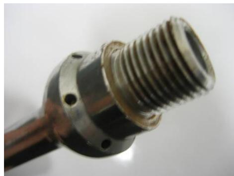
side view of pilot pin showing vac holes
