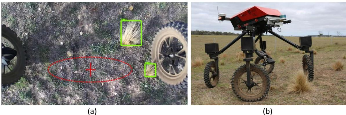
**Fig. 5.** (a) A sample detection frame from the downwards-looking camera with the spray target position marked by a red cross, the spray coverage area marked by a red oval and the weed detections by green bounding boxes.
