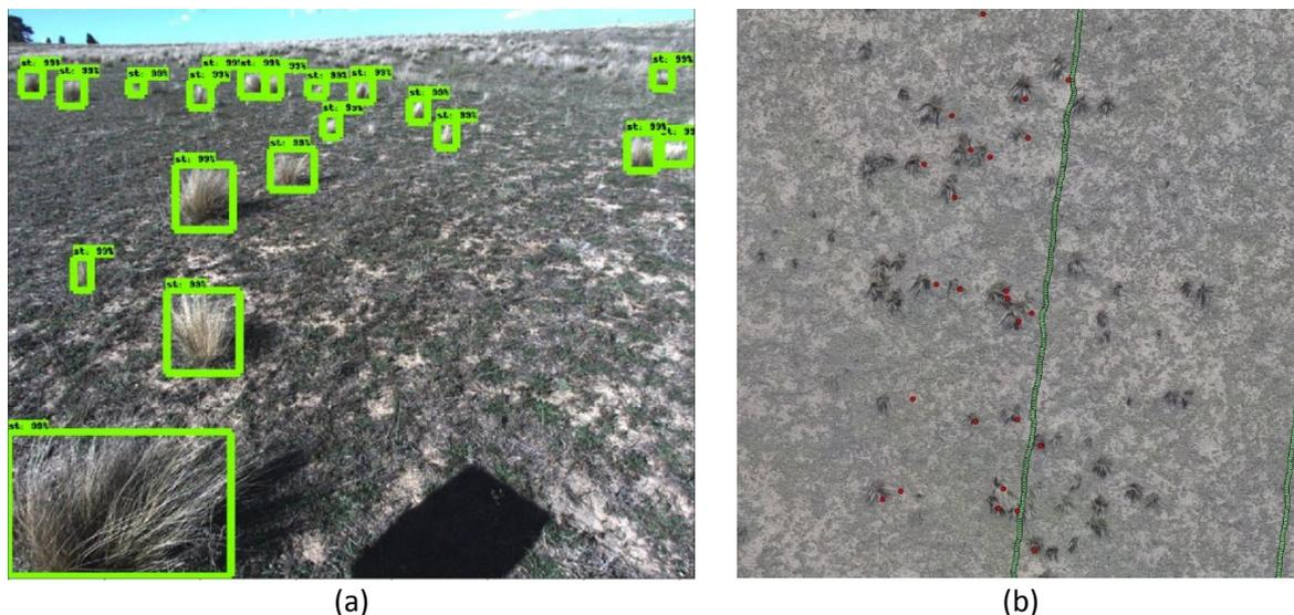
**Fig. 4.** (a) The output of automated serrated tussock detection software showing green bounding box detections and confidence levels. Data was collected at Arthursleigh using SwagBot’s forward facing camera. (b) A sample region showing high-resolution (1cm per pixel) aerial orthomosaic (data collected using 3DR Solo drone), SwagBot track (green) and weeds detected by SwagBot (red). The georeferenced weed locations correspond well with the aerial imagery, with only a small offset observed.
