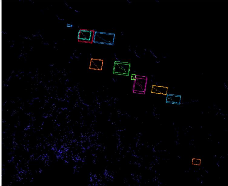
**Fig. 11.** Clustering of the 3D point cloud into 'unknown' objects. These can then be identified as cattle using the 2D detections.
