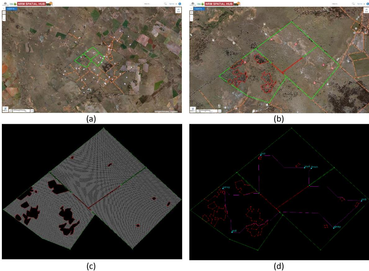
**Fig. 2.** (a) Figure showing the Chatswood property boundary (black lines), internal paddock boundaries (orange lines) and water points (white circles) in FarmMap4D. (b) SwagBot permissive areas (green lines) and restrictive areas (red lines) defined in FarmMap4D. (c) Mesh used by the autonomous path planning algorithm. (d) SwagBot mission plan showing route (magenta dashed line) and waypoints (cyan circles).
