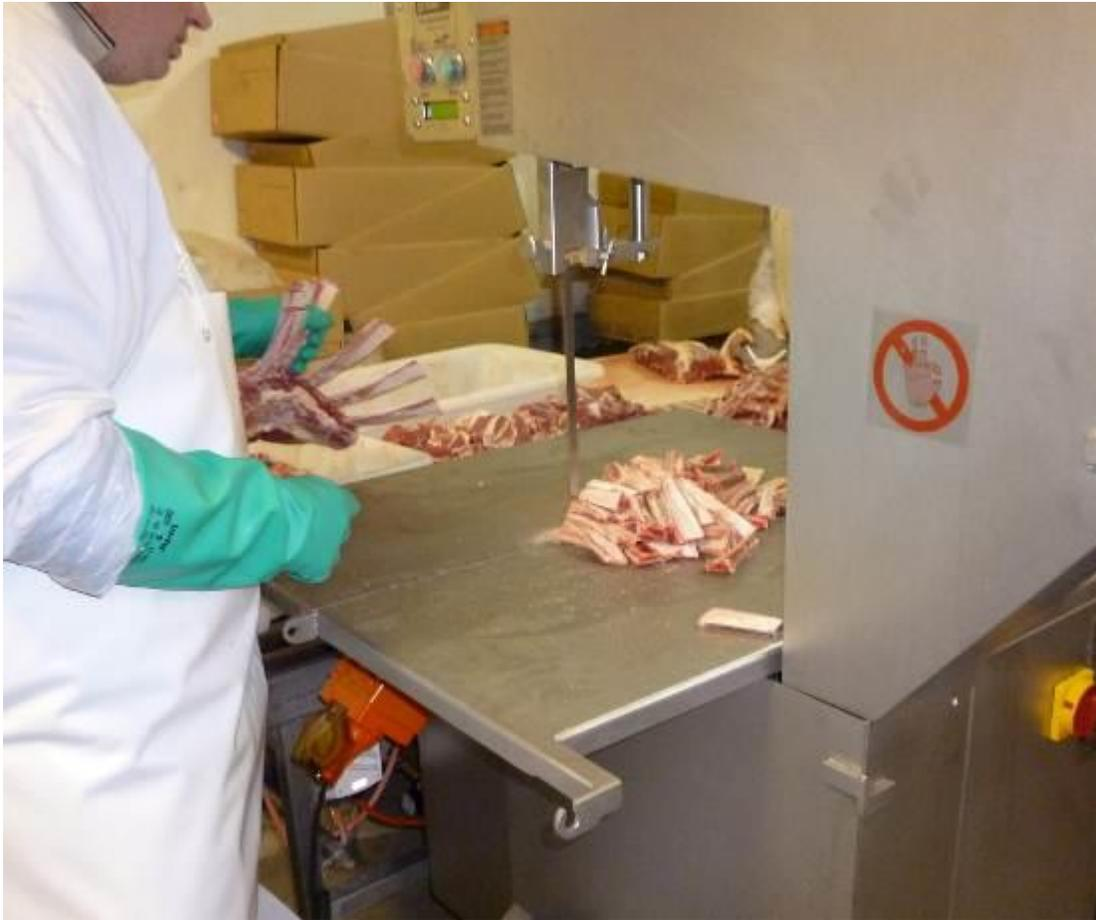
**Fig.24 Bladestop in use at NCMC**
