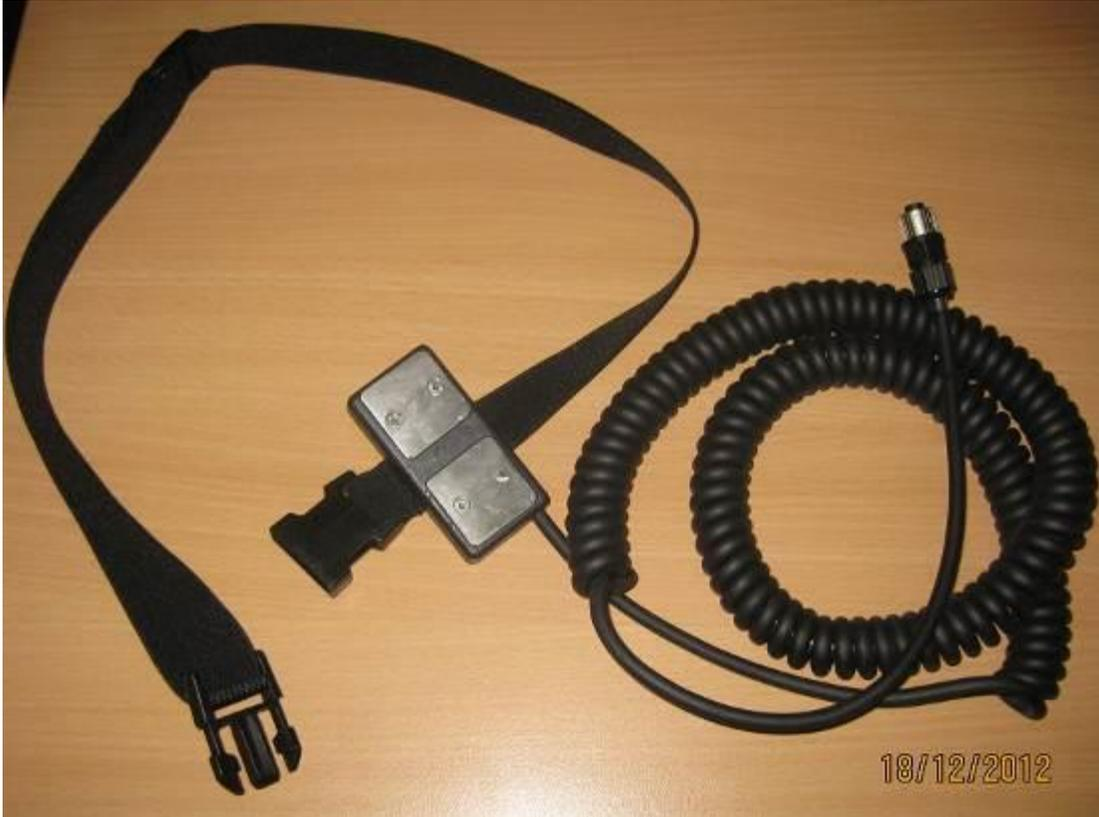
**Fig.17** Images showing the new waist strap design including Contact Block, elastic waist strap, cable and new connector
