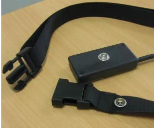
**Fig. 19 Press Stud connection of Contact Block to elastic strap**
