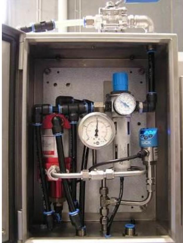
**Fig.5 Air intensifier installed into the ACC saw**
