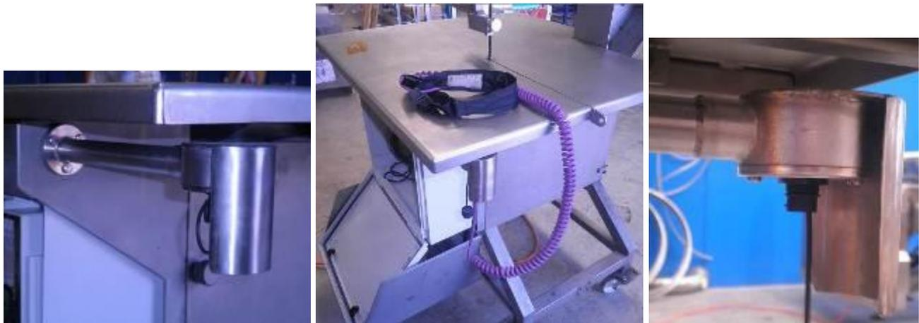
**Figs. 16 Connection point for waist strap to saw.**
