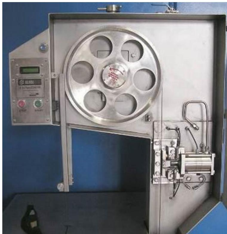
**Fig.4 New Bladestop mechanism installed into the ACC saw**
