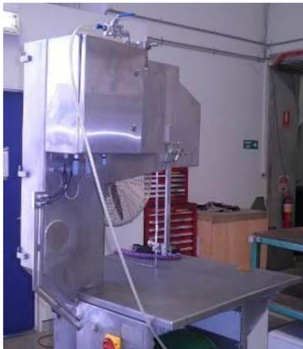
**Fig.6 Air intensifier stainless steel box installed on the ACC saw**
