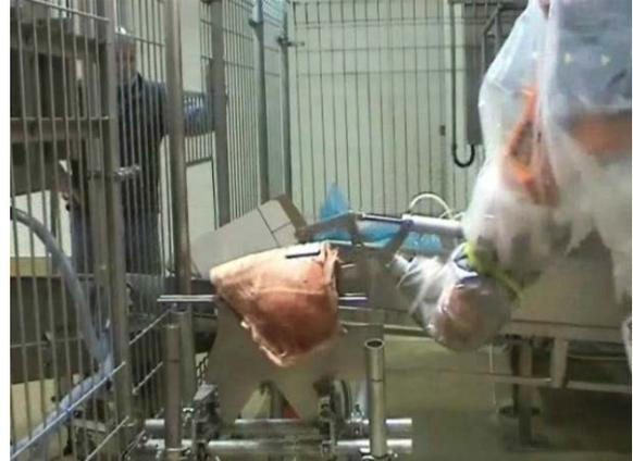
Step 2 – Integration robot transfers the middle section to the middle system loading fixture on the middle system carousel
