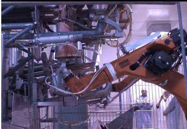
Step 1 – Primal system (Tower 2) removes middle/saddle from carcase (after forequarter has been removed in the first primal tower)
