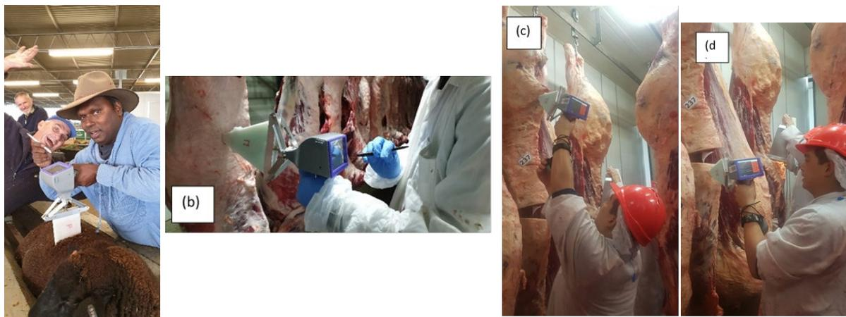
Figure 6 The proposed Microwave System used for various measurement (a) Live sheep measurement at feedlots (b) Lamb carcass measurement at abattoir (c) Beef carcass P8 fat depth measurement at abattoir (d) Beef carcass Rib fat depth measurement at abattoir
