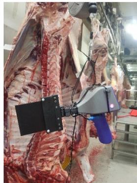
Figure 7 Beef carcass hot P8 and Rib fat depth measurement at abattoir kill floor using a spring balancer.
